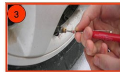
Jack or hoist the vehicle up, then remove valve core, completely deflate tire with valve at bottom of wheel assembly
